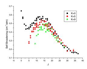
790 self-broadening coefficients have been measured for 0 < J < 34 and 0 < K < 12 values using a multispectrum fitting procedure [4].
